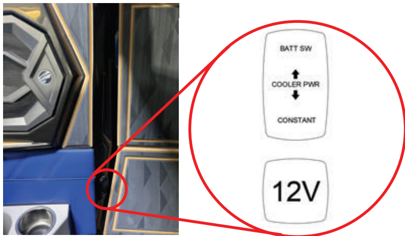
Image 13: Ultré Chill Outlet Toggle Switch
